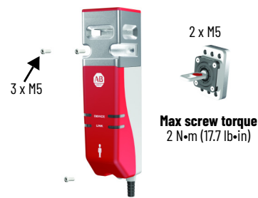
Figure 2 - Required Mounting Hardware for Switch and Actuator
