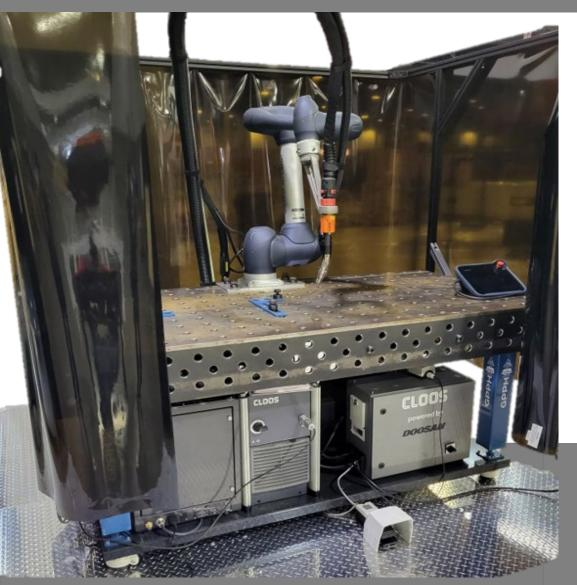
**ArcBoT** by **CLOOS** comes complete and ready for your move to automated welding – all components perfectly matched in a compact `Ready to Weld` production arc-welding package.
